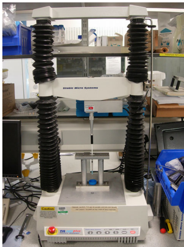
Fig. 4 Texture analyser apparatus used for injectability studies
